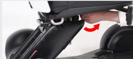
Hold the armrests on both sides of the seat and lift it upward, leaving the seat a way from the base.
